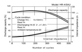
If a battery is charged at a current higher than the prescribed current level, or over-discharged to the point of polarity reversal, or used at low or high temperatures exceeding the recommended range, the charge/discharge cycle life will decrease.
