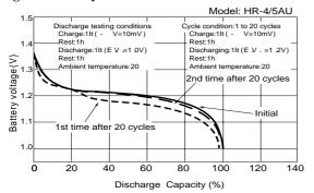
Therefore, if a device is designed so that the discharge end voltage is high, or if the device is used in such a way that shallow discharge occurs repeatedly, the memory effect may result, and for this reason we recommend explaining the method for eliminating the effect in operation manuals.
