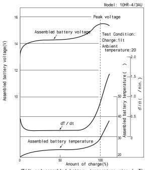
dT/dt and assembled battery temperature rise ( T) vary depending on such conditions as ambient temperature, insulating properties of the assembled battery case, and generation of heat from the device in which the batteries are used. Therefore, the device must be used to determine the most suitable values.
