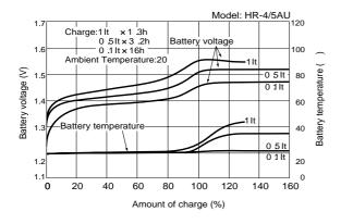
Fig.8 Charge temperature characteristics
