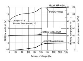
Also, as there is a limit to the negative electrode's ability to consume oxygen gas formed at the positive electrode due to over-charging, a maximum allowed charging current has been set to assure a balance between the amount of oxygen gas formed and the negative electrode's ability to consume it.
