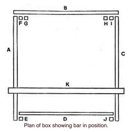
A, B, and C are the sides, each consisting of six boards each 4 ft. x 6 in. x 1 in., nailed to the uprights half an inch apart to allow ventilation.
