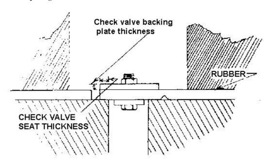
Check valve backing thickness in inches
