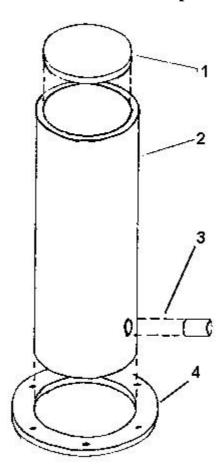
Welded hydram: accumulator: exploded view
