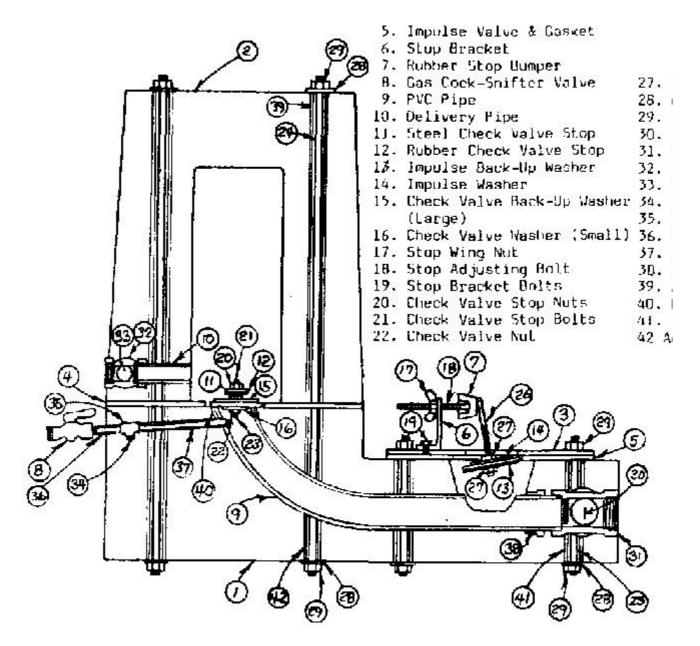
Exploded view of 2 - piece concrete hydram
