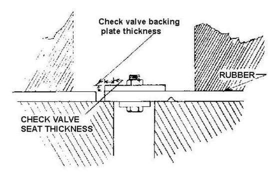
Check valve backing thickness in millimeters
