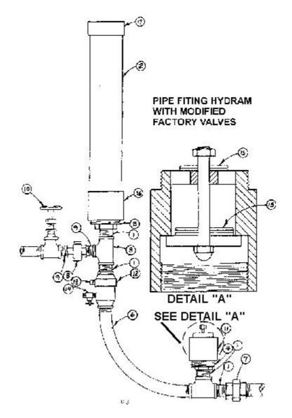
Pipe fitting hydram with modified factory valves
