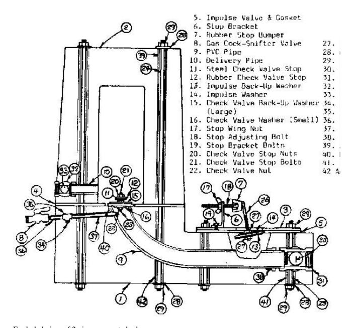
Exploded view of 2 piece concrete hydram
