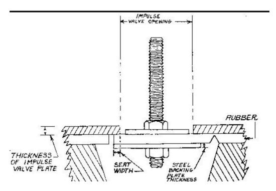
Impulse valve steel backing
