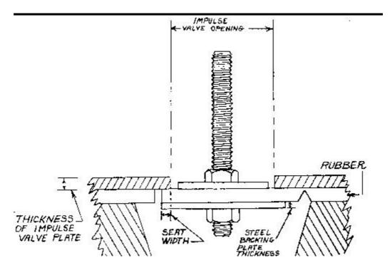
Thickness of the impulse valve plate in millimeters
