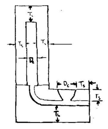
Concrete hydram design parameters
