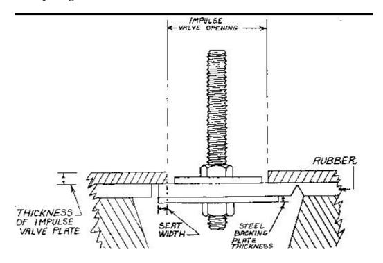
Impulse valve steel backing - metric
