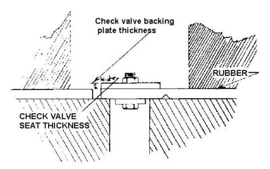
Check valve backing thickness in inches
