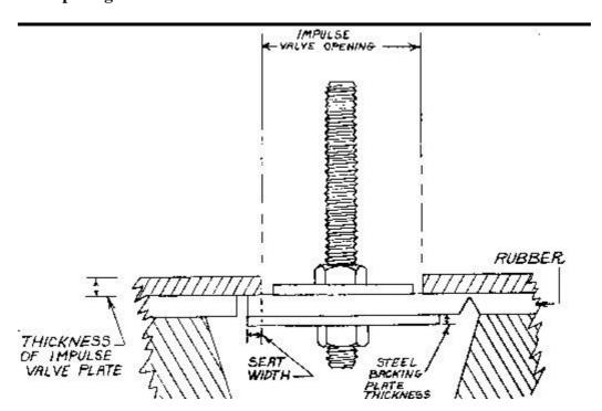
Impulse valve seat width in millimeters
