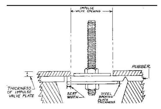
Impulse valve steel backing
