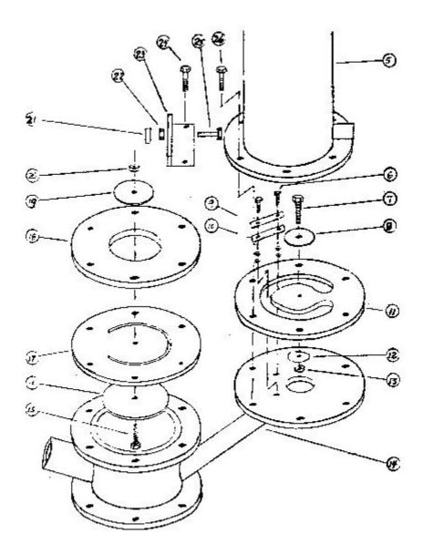
Welded hydram: exploded view
