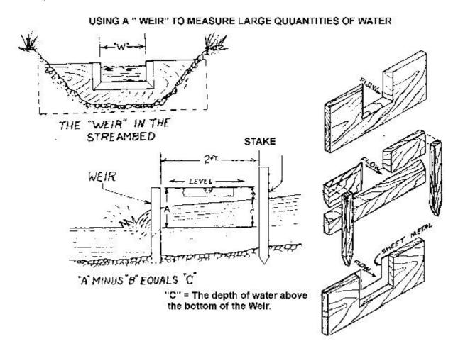
Using a "weir" to measure large quantities of water
