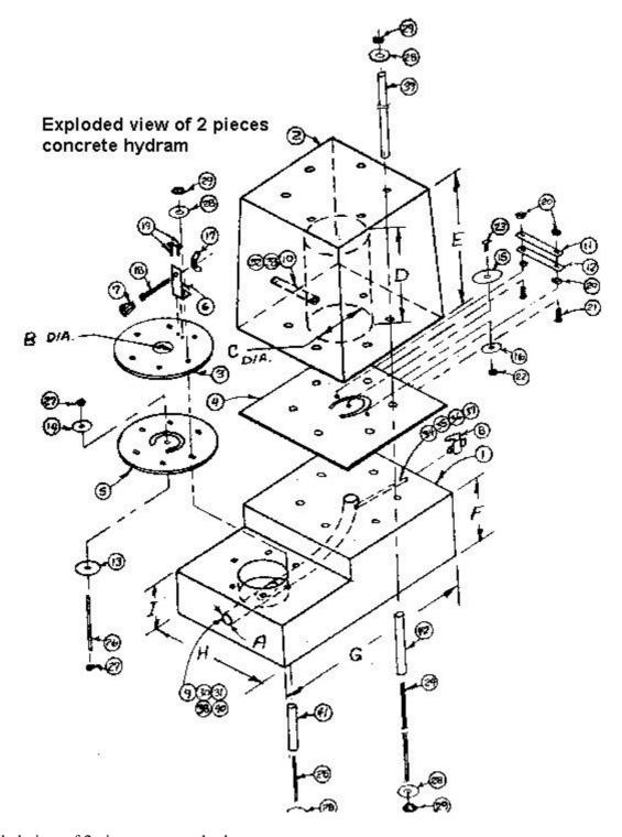
Exploded view of 2 piece concrete hydram
