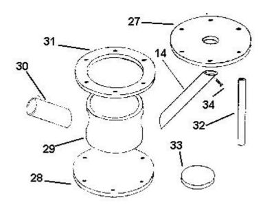
Welded hydram, impulse cavity: exploded view
