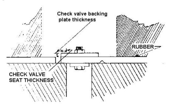
Check valve backing thickness in millimeters
