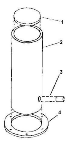
Welded hydram, accumulator: exploded view
