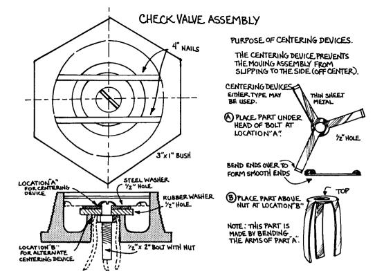
a bit of clearance for the water to pass. Drill two holes on each side of the middle for a 4" common nail to pass just above the valve metal washer, to keep it in place. Leave enough clearance so the valve can open just about 1/16". Spread the bolt with a centre punch just below the nut, so the nut can't work loose. Cut the nails off and file threads across their ends so the bushing will screw into the tee above it
