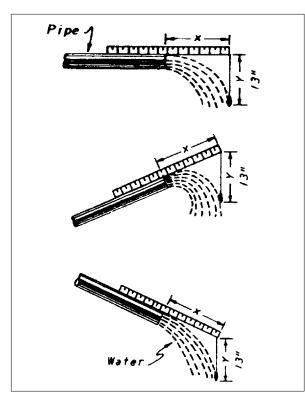
*Figure 1.—Measuring horizontal distance (X) of a pipe flowing full with vertical drop Y=13".*
