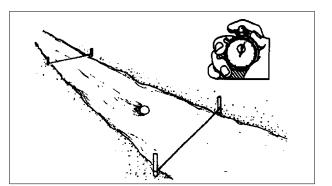
*Figure 2.—Measuring the flow rate in a stream or channel by timing a float.*
