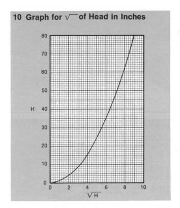
the square root of 27 to be about 5.2. Substituting the values in the equation  $Q = K\sqrt{H}$ , Q is calculated to be 806.0 (5.2 x 155).
