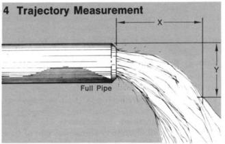
I ne trajectory method of water measurement is a form of velocity area calculations that can be used for determining the rate of flow discharging from a horizontal pipe flowing full. Two measurements of the discharging jet are required to calculate the rate of flow of the water. The first measurement is the horizontal distance, "X", (parallel to the centerline of the pipe) required for the jet to drop a vertical distance "Y" which is the second measurement.
