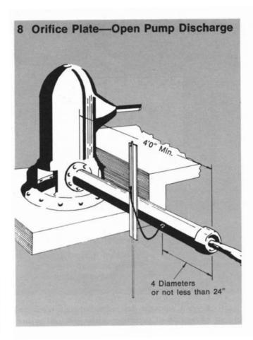
K = a constant dependent upon a combination of pipe size, orifice size and orifice shape, and discharge conditions. H = Head in inches.
