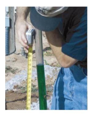
Figure 8. Two photos showing how to measure the head (ft) in a gated pipe system. The head is the distance between the water level in the tube and the center of the pipe. These are Rite-Flow<sup>TM</sup> gates and there is about 3 ft of head. According to Table 8, the flow is approximately 39 gpm per gate.
