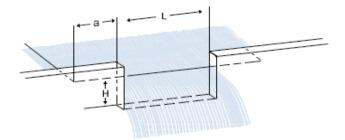
Figure 4. Diagram of a rectangular weir where L = width of weir opening (4 to 8 times H), H = head of weir (measured 6 ft upstream of weir) and a = at least 3\*H.
