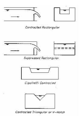
Figure 3. Diagrams of various types of weirs used to measure flow rate in an open ditch. (USDI-BOR, 1997).
