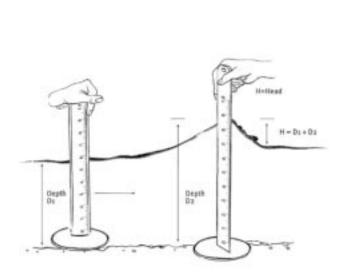
Figure 2. Using a velocity Rod. (Waterwatch, 2002).
