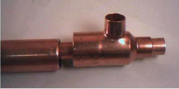
The heat exchanger is made up of two pipes one on the inside of the other. Steam flows down the center .5 inch inner pipe being cooled by water held around this by a 1 inch outer pipe. The end caps are 1" x .5" x .5" copper "T" fittings with the ridge filed off on the inside so the .5 inch pipe slips completely through it. The 1 inch pipe is 20 inches long and the .5 inch is 25 inches long. This or longer will work fine.
