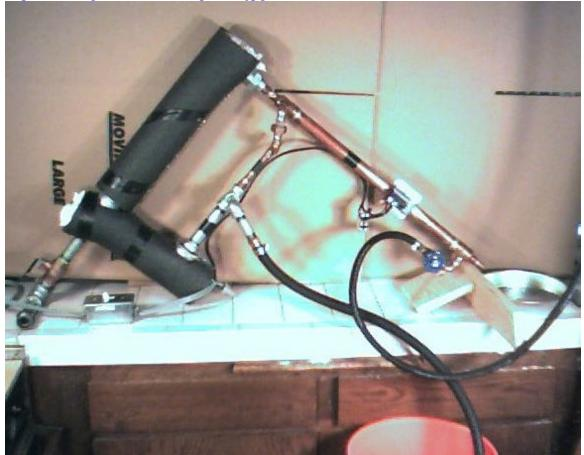
Use insulation like shown in the picture to keep the heat in. This adds about 5 percent to the efficiency of the unit.
