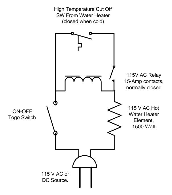
If the cooling flow stops then the temperature switch will turn off the current flow to the heater element. If the water flow stops totally then about 40 sec latter the 150 degree F
