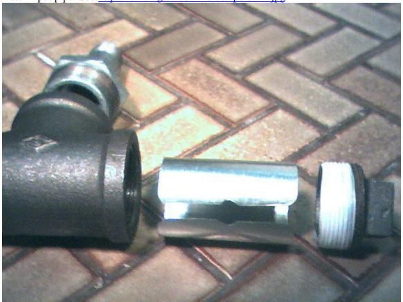
The insert is made of sheet metal. The hole and slot is positioned near the bottom.
