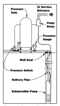
Figure 1: Components of the "demand" type system.
