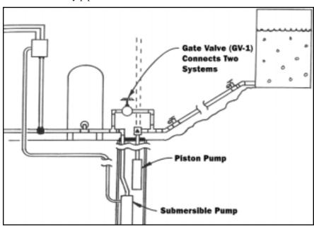
Figure 2: Demand and store type systems joined in a side-by-side method.
